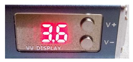
Until the voltage setting is displayed pressing of either the **V+** or **V-** will have NO effect.
