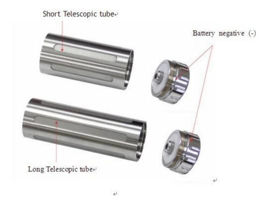
There are two telescopic tubes available for the iTaste SVD. The short tube supports 18350 batteries and long tube supports stacked IMR 18350(2), 18500 and 18650 batteries. You can use 2 IMR high drain 18350 batteries at the same time, which will give you the full arrange of voltages/Wattages and proper power needed to use the device.
