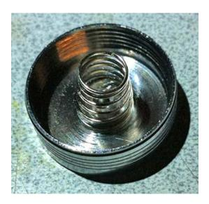
Later versions will be provided with an uprated spring – in the meantime you can retrofit any suitable spring from a cheap torch to rectify any problems you may encounter regarding flat headed 18650 batteries like so;
