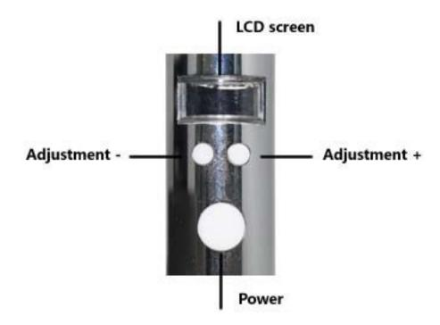
Note: when a battery is inserted the screen may flash once and then turn off – the device is not yet turned on – you will need to click the power button 5 times to turn the device on.
